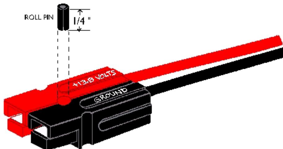
Housings should be mated according to the diagram above, viewing from the contact side (opposite the wire side), tongue down, hood up, RED on the LEFT, BLACK on the RIGHT. Use a
